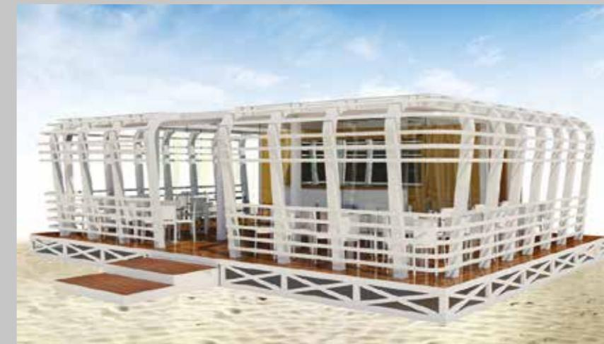
*Integrated project for a prefabricated beach club. Steel or wood structure with retractable roof.*
